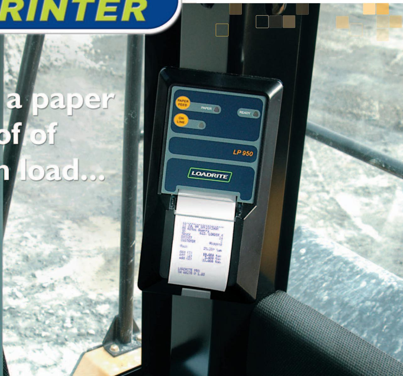
Add a Loadrite Printer to your Loadrite Weighing System and get a hard copy proof of each load. The Loadrite Printer is a direct plug-in accessory for the entire range of Loadrite Onboard Weighing Systems. It delivers time-stamped and dated hard copies of weighing information, including each bucket load and the total load. The printer is robust and reliable, with proven performance in extreme environments around the world.
